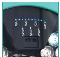
Adjustable light intensity with touchless infrared sensor
